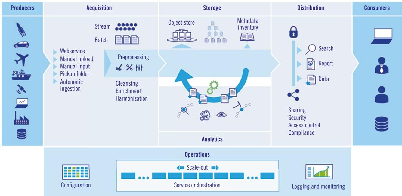
FIGURE 2 Function-oriented structure of a toolchain (© Werum)
